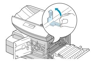
**6** Turn the jam remove lever back to the original position.
